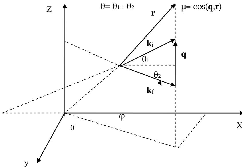
Fig. 1 Impulses of incident ( $\mathbf{k}_i$ ) and scattering ( $\mathbf{k}_f$ ) particles in three- dimensional coordinate system with the transfer impulse  $\mathbf{q} = \mathbf{k}_i - \mathbf{k}_f$ .
