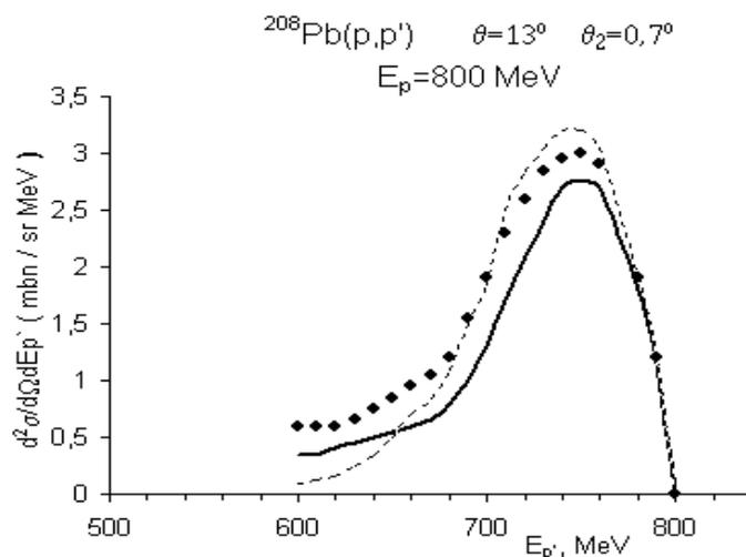
Fig.2 Dependence of the double differential cross section at energy of incident protons 800 MeV, scattering angle  $\vartheta = 13^\circ$  for nuclear  $^{208}\text{Pb}(p, p')$  on the energy of the scattered protons, solid line-the obtained results, points - experimental data [9], and a bar line – the theoretical calculations obtained in [12].
