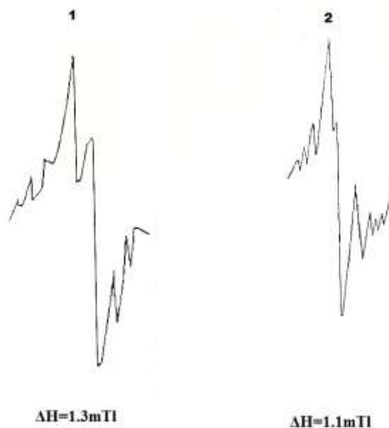
Fig. 5 EPR spectrum of unsaturated elastomers with sensitizer DSCB irradiated by dose 500kGy in cold conditions 77K. 1. The spectrum of irradiated elastomer cis-SKB in the presence of 8 parts DSCB. 2. The spectrum of irradiated elastomer SKN-26 in the presence of 8 parts DSCB.
