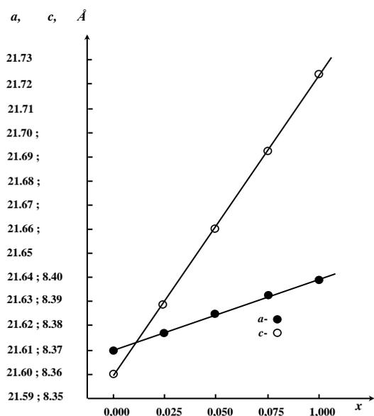
Fig. 1. Dependence of crystal lattice parameters of  $Cu_{1.80-x}ZnTe$  monocystals on the x.
