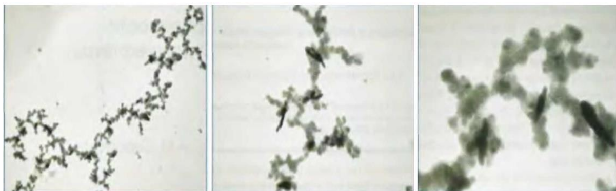
Fig. 2. Pictures of paraffin samples taken from Transistor Electron Microscope.
