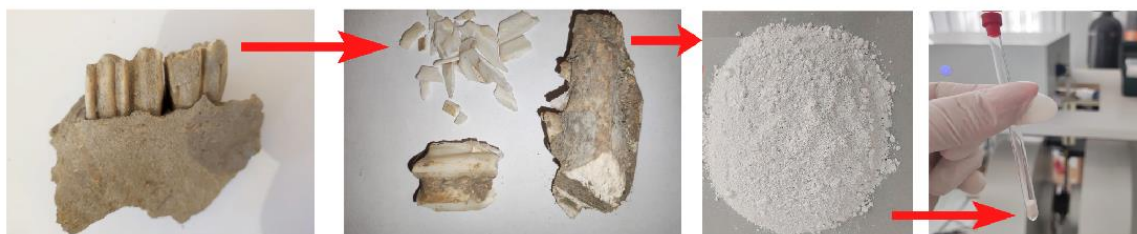
Fig. 1. Tooth sample preparation for ESR dating.
