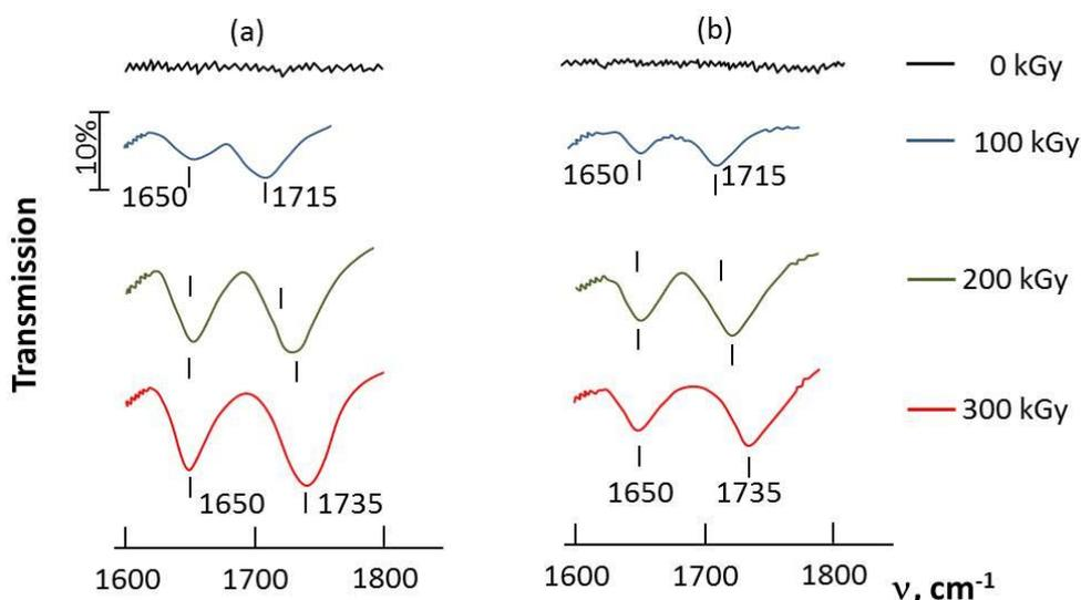
Fig. 3. FTIR transmission spectra of HDPE polymer (a) and HDPE/GaAs (b) composite films, irradiated with gamma absorption doses of 100, 200, 300 kGy, in frequency range  $\nu = 1600\text{--}1800$   $\text{cm}^{-1}$ .
