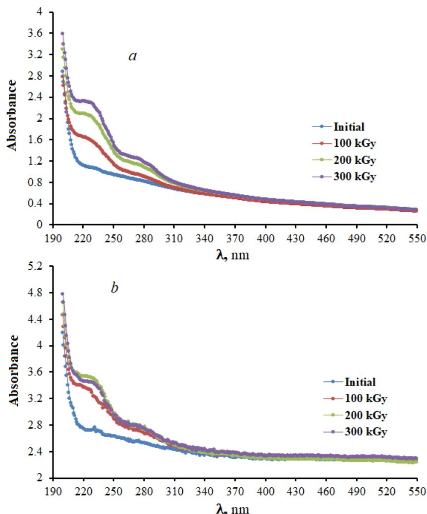
Fig. 1. Absorption spectra of the initial and gamma-irradiated HDPE polymer (a) and HDPE/GaAs composite (b) films.
