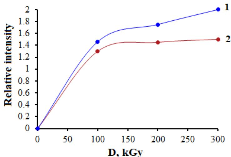
Fig. 2. Dose dependence of the intensity of optical absorption band at  $\lambda = 280$  nm. 1 – HDPE and 2 – HDPE/GaAs.
