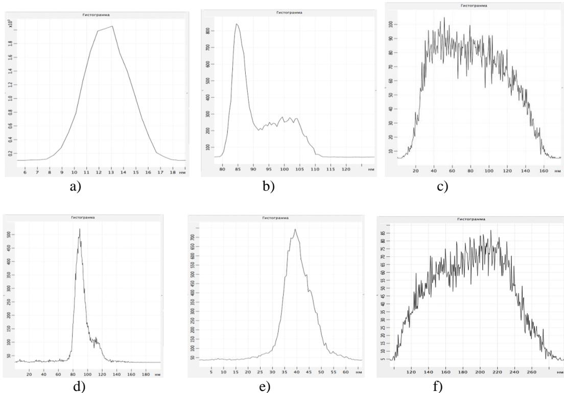
*Fig. 3. Figure 3. Histograms of GaSe monocrystals: a — initial sample; b — initial + thermally annealed at 100 °C for 60 minutes; c — irradiated at 0.5 kGy; d — irradiated at 1 kGy; e — thermally annealed at 100 °C for 60 minutes + irradiated at 0.5 kGy; f — thermally annealed at 100 °C for 60 minutes + irradiated at 1 kGy.*
