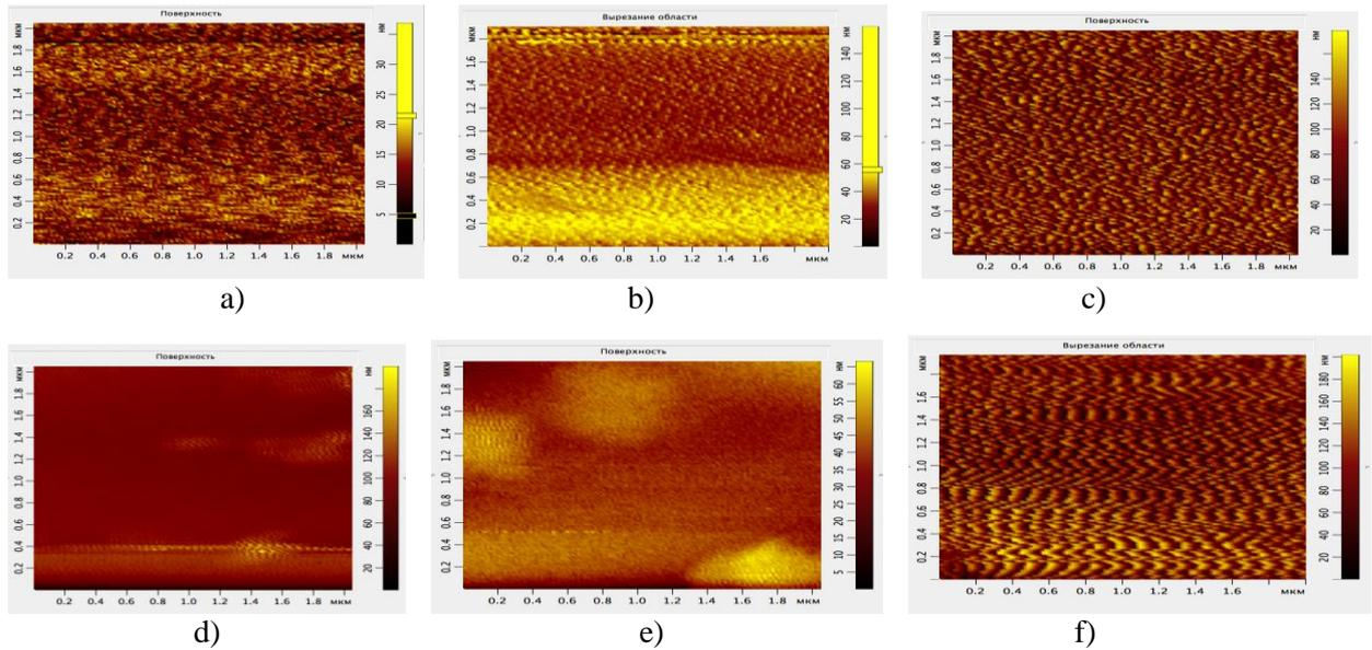
*Fig. 1. 2D Surface Images of GaSe Monocrystals Captured by Atomic Force Microscopy (AFM): a — initial (untreated) sample; b — initial sample after thermal annealing at 100 °C for 60 minutes; c — sample irradiated at 0.5 kGy gamma dose; d — sample irradiated at 1 kGy gamma dose; e — thermally annealed (100 °C, 60 min) and irradiated at 0.5 kGy gamma dose; f — thermally annealed (100 °C, 60 min) and irradiated at 1 kGy gamma dose.*
